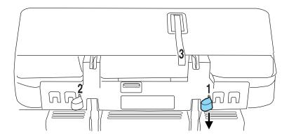
6. From the rear of the vehicle, fold seat back by  $\mathbf{pulling}$  and  $\mathbf{releasing}$  the number 1 strap.
